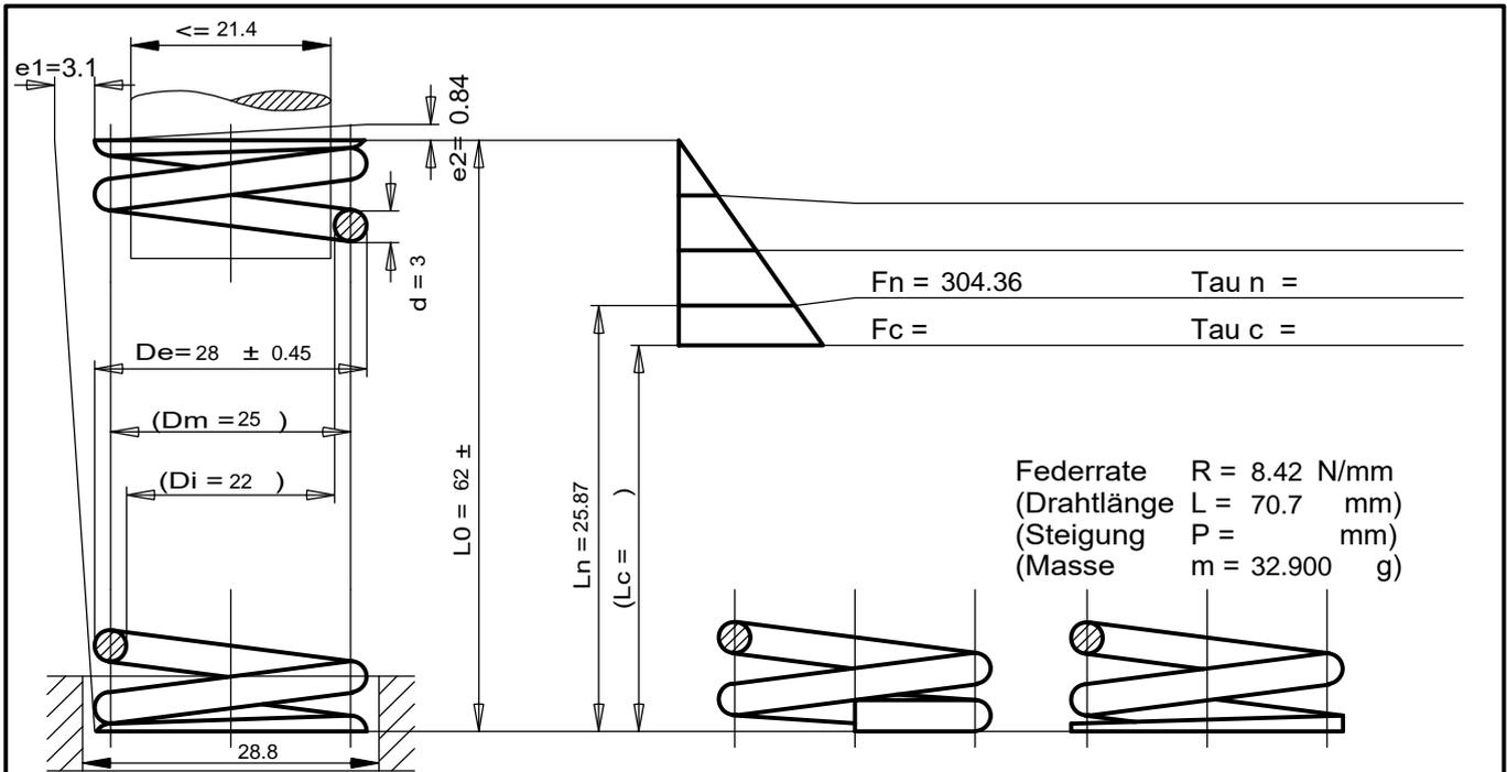
Federrate  $R = 8.42 \text{ N/mm}$
