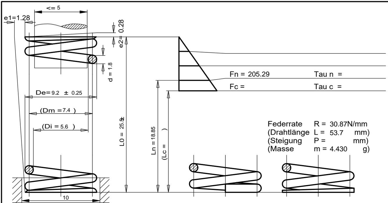
Federrate  $R = 30.87\text{N/mm}$
