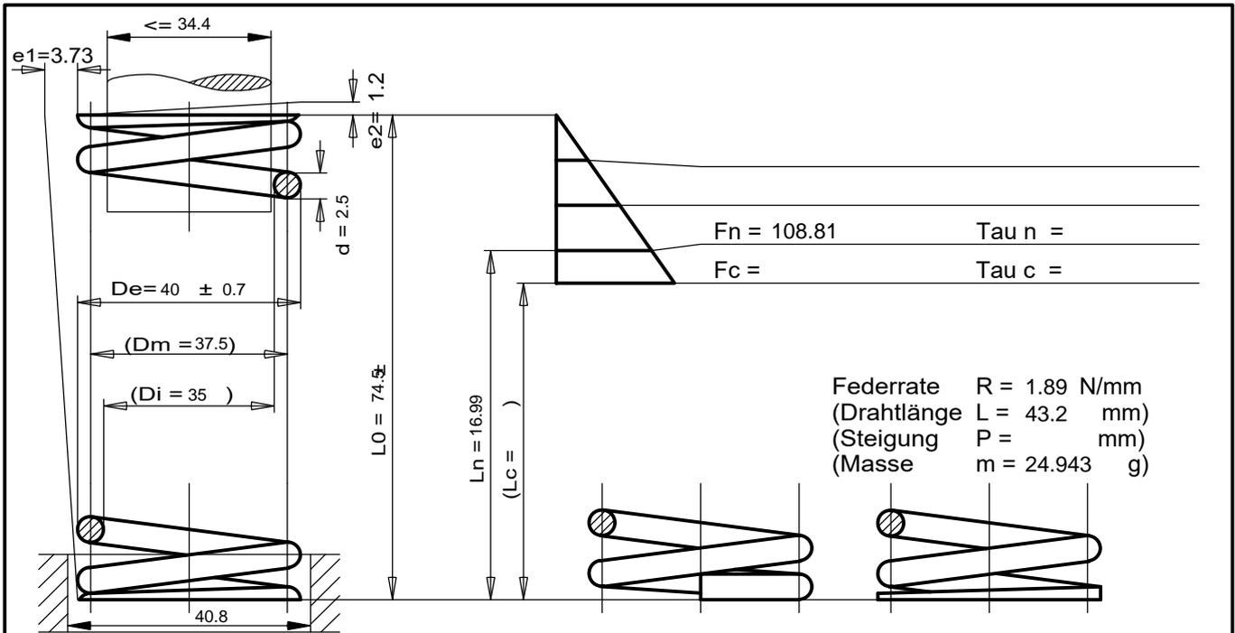
Federrate  $R = 1.89 \text{ N/mm}$
