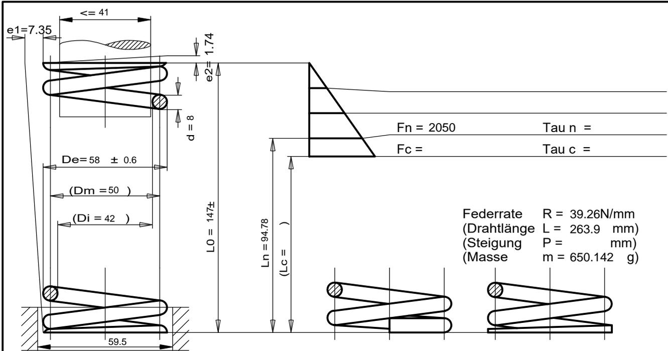
Federrate  $R = 39.26\text{N/mm}$
