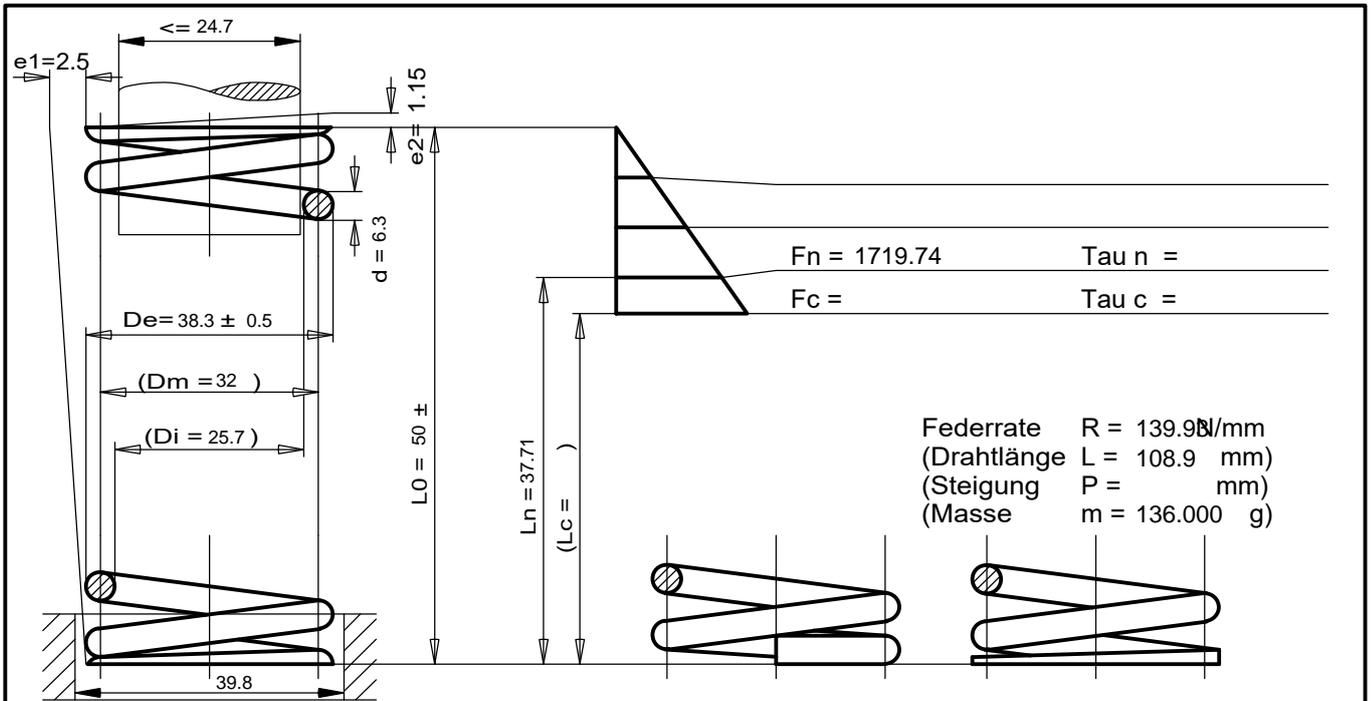
Federrate  $R = 139.9 \text{ N/mm}$
