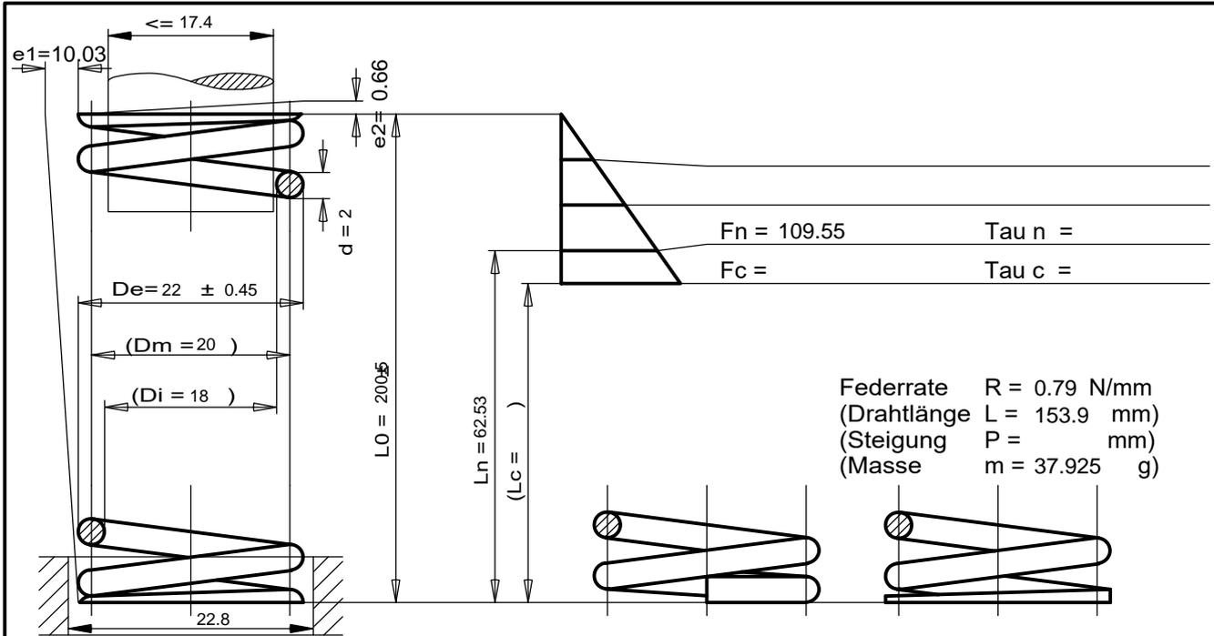
Federrate  $R = 0.79 \text{ N/mm}$
