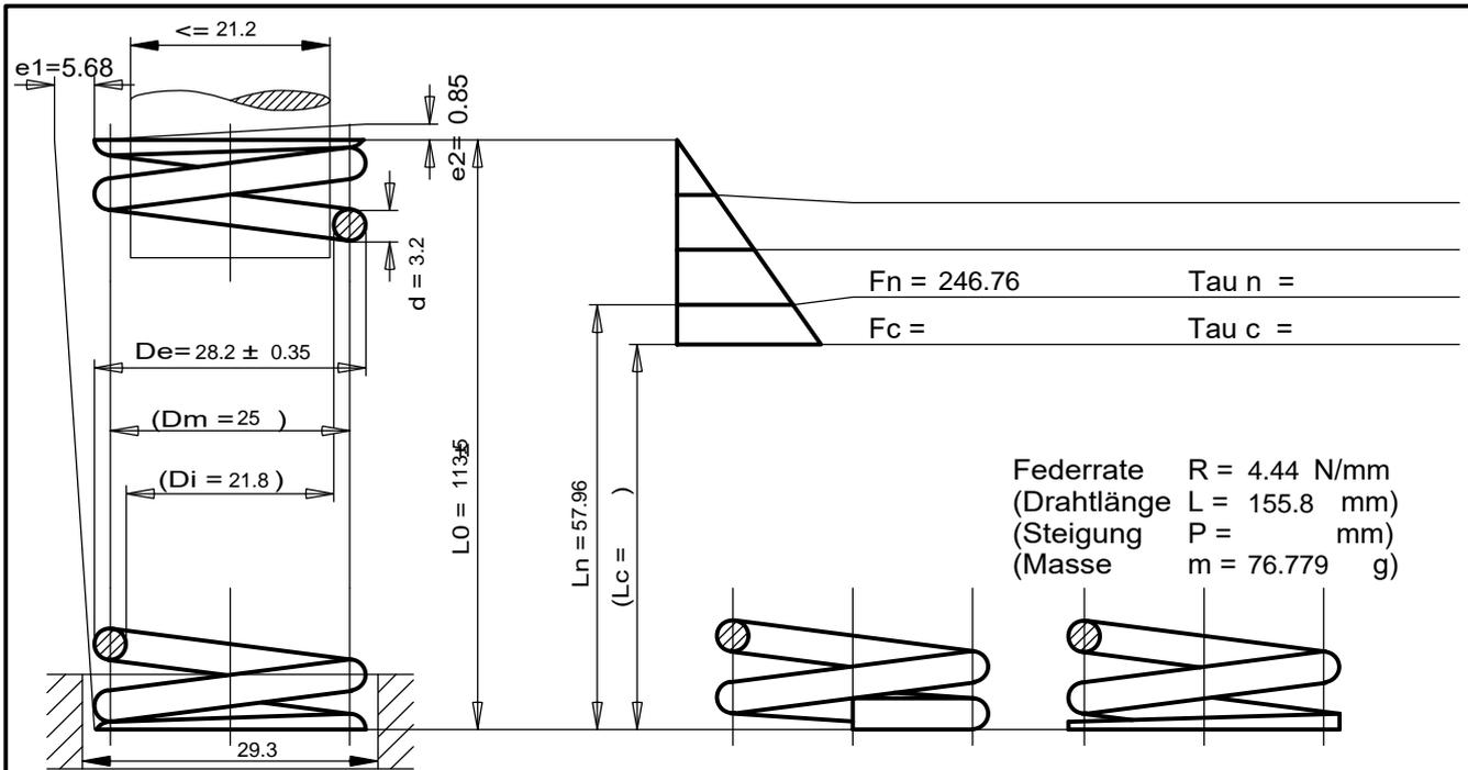
Federrate  $R = 4.44 \text{ N/mm}$
