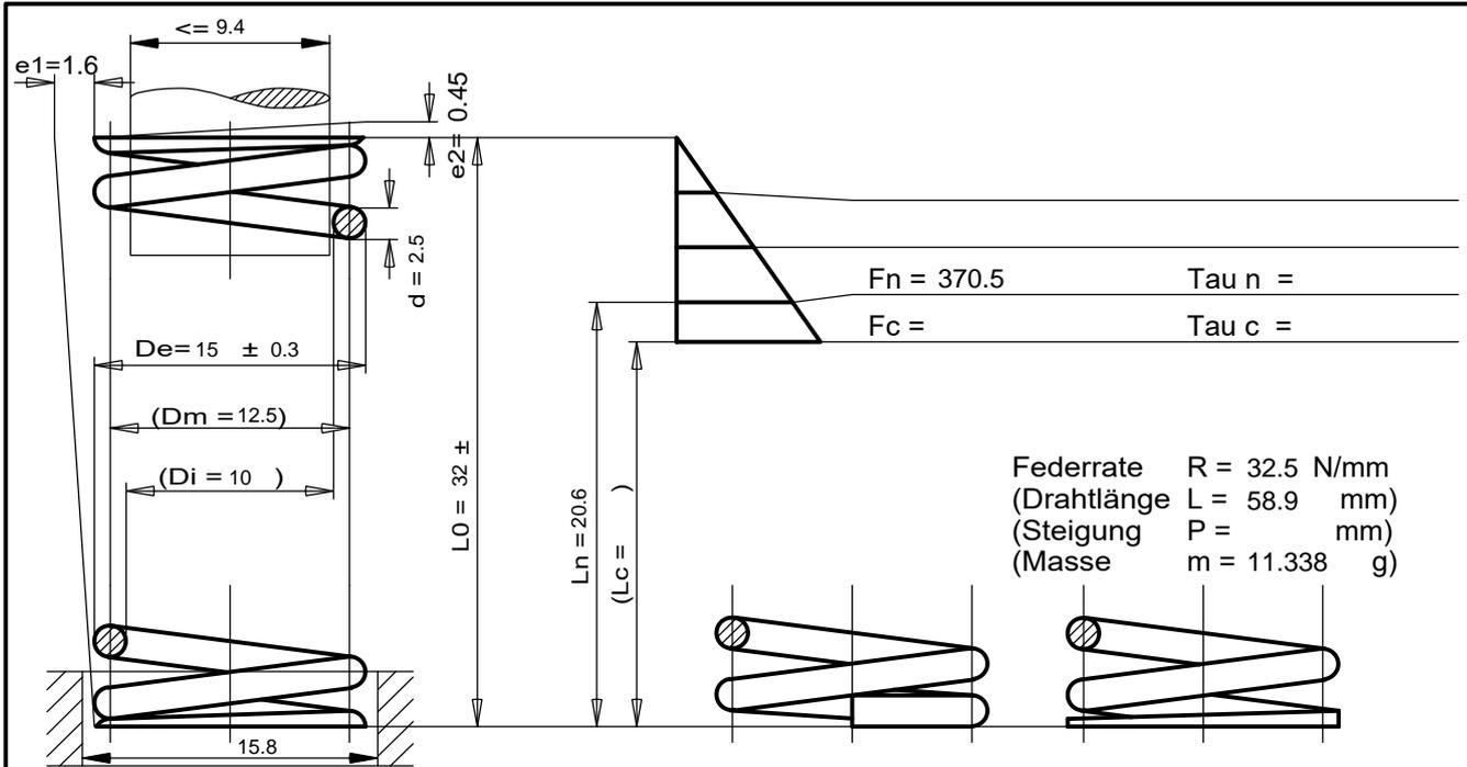
Federrate  $R = 32.5 \text{ N/mm}$
