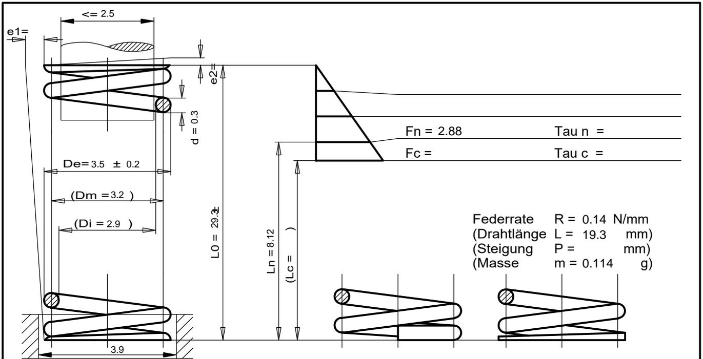
Federrate  $R = 0.14 \text{ N/mm}$
