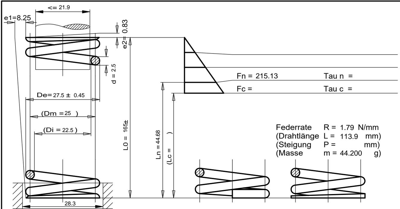
Federrate  $R = 1.79 \text{ N/mm}$
