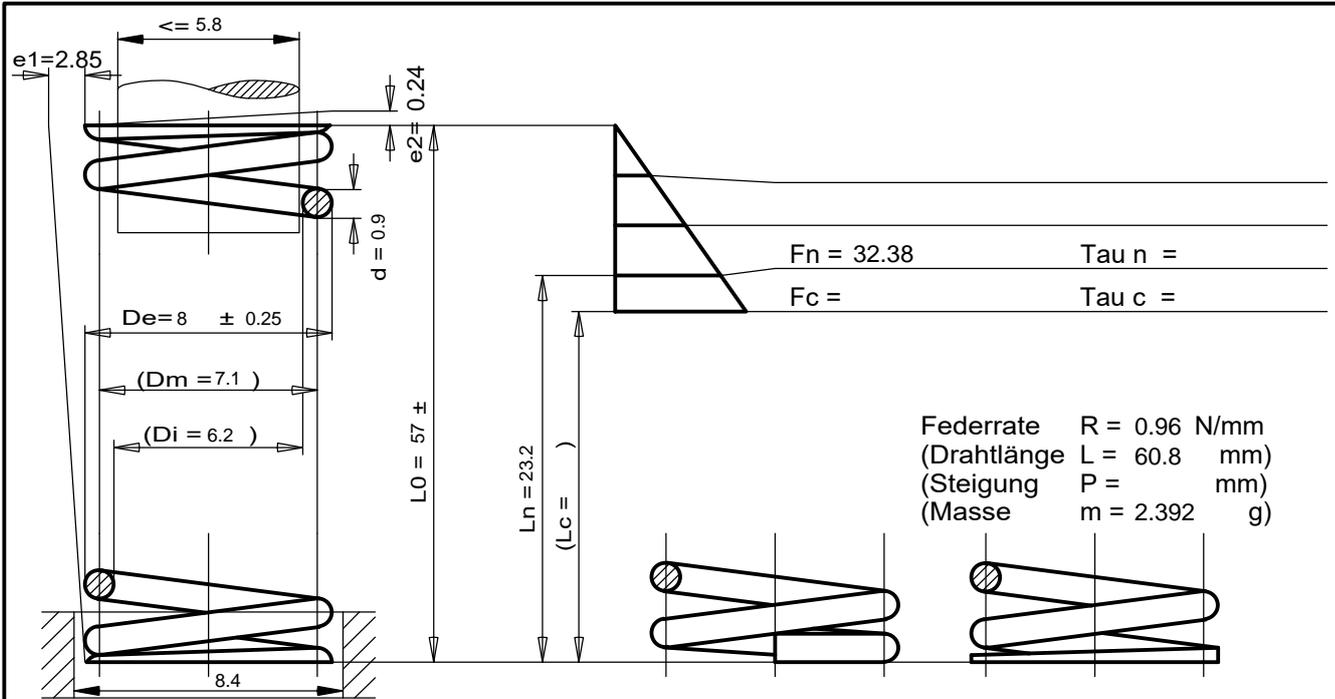
Federrate R = 0.96 N/mm
