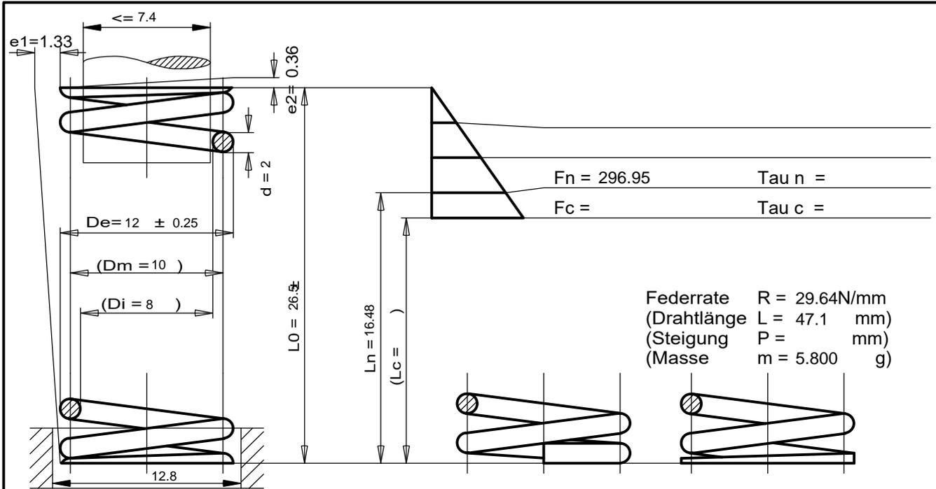
Federrate  $R = 29.64 \text{ N/mm}$
