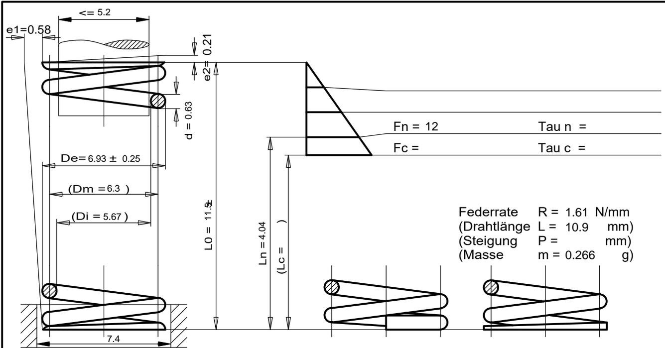
Federrate  $R = 1.61 \text{ N/mm}$
