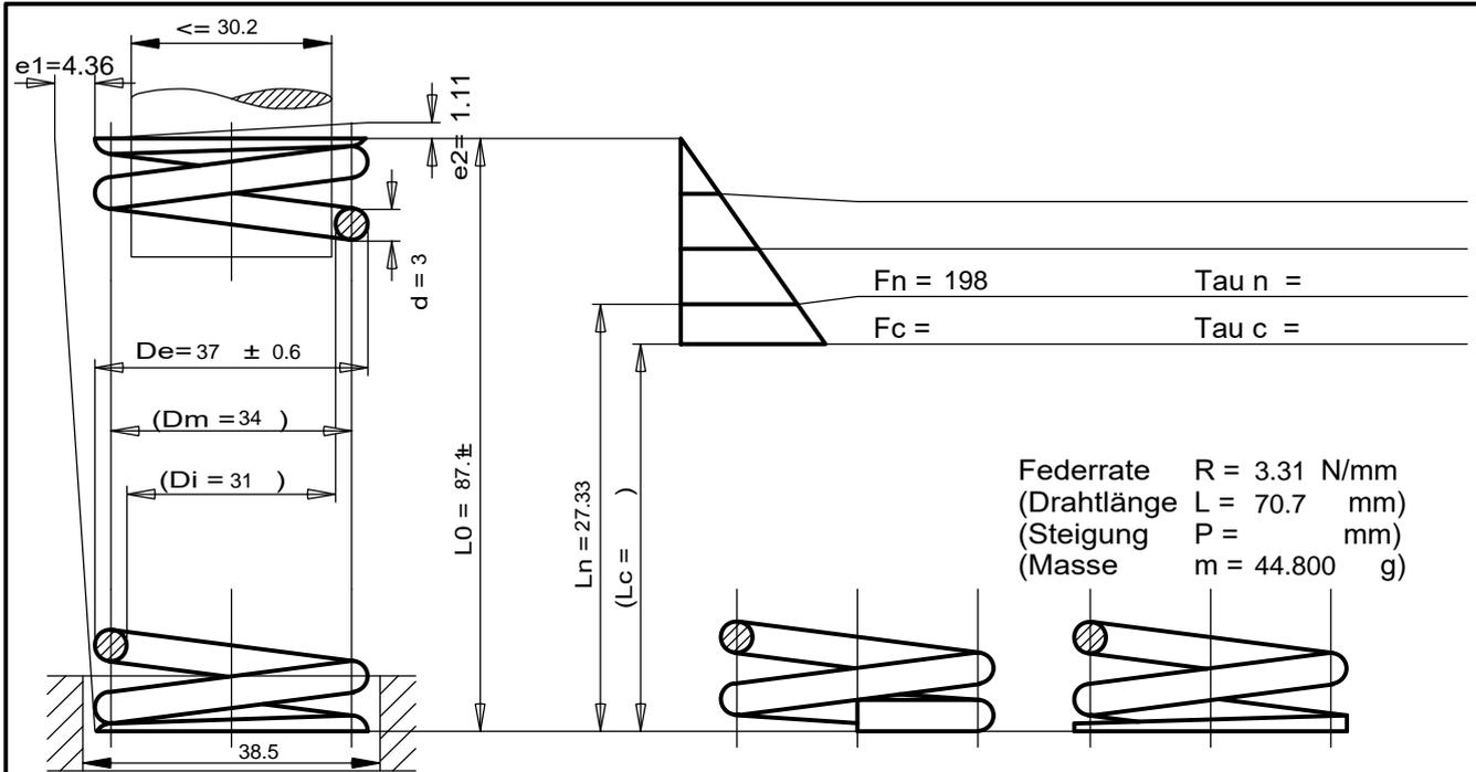
Federrate  $R = 3.31 \text{ N/mm}$
