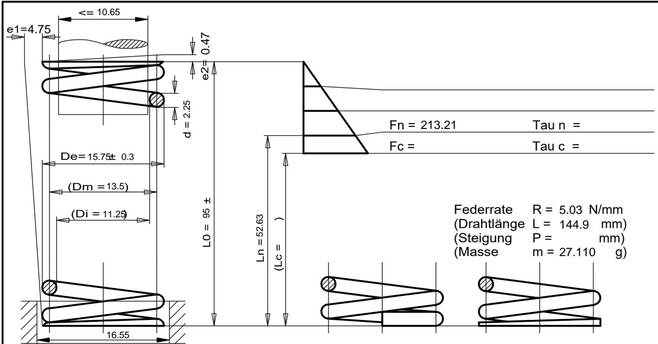
Federrate  $R = 5.03 \text{ N/mm}$
