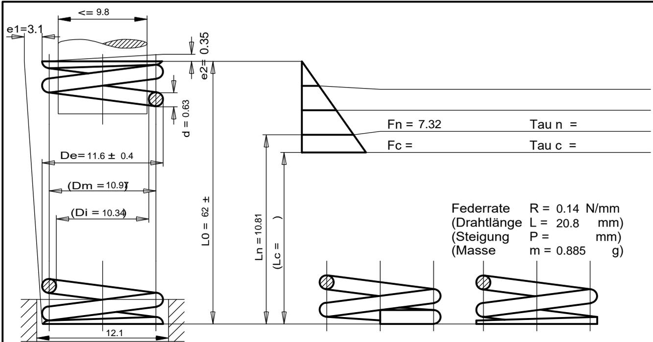
Federrate  $R = 0.14 \text{ N/mm}$
