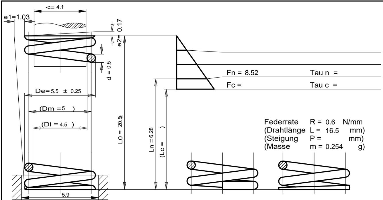
Federrate  $R = 0.6 \text{ N/mm}$
