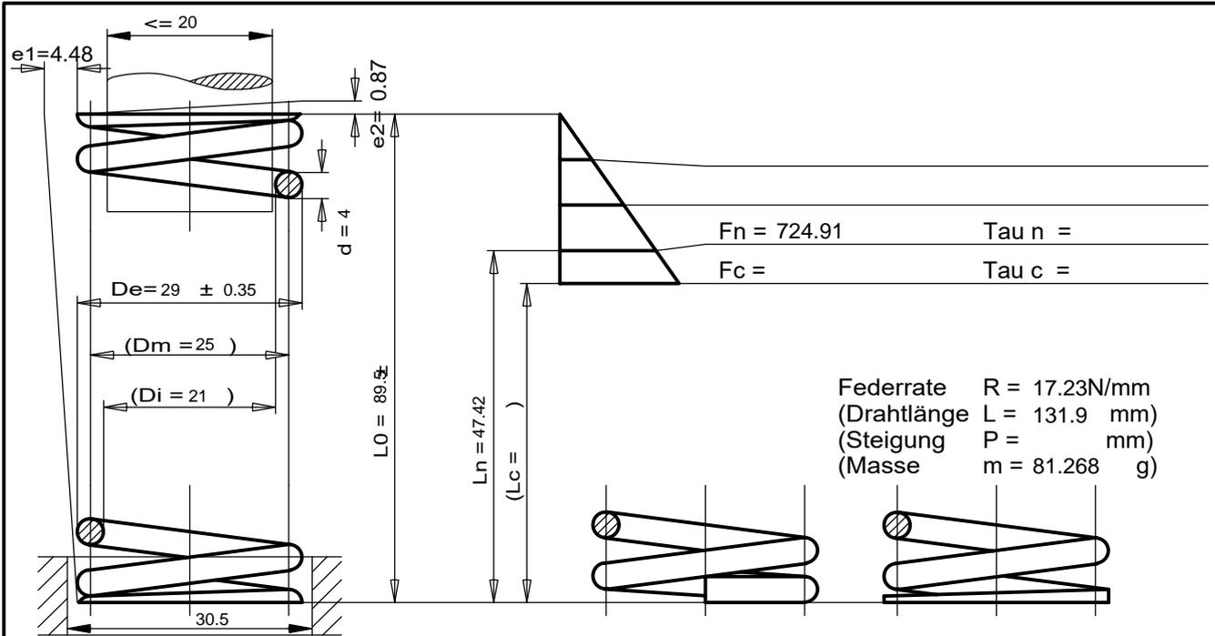
Federrate  $R = 17.23 \text{ N/mm}$
