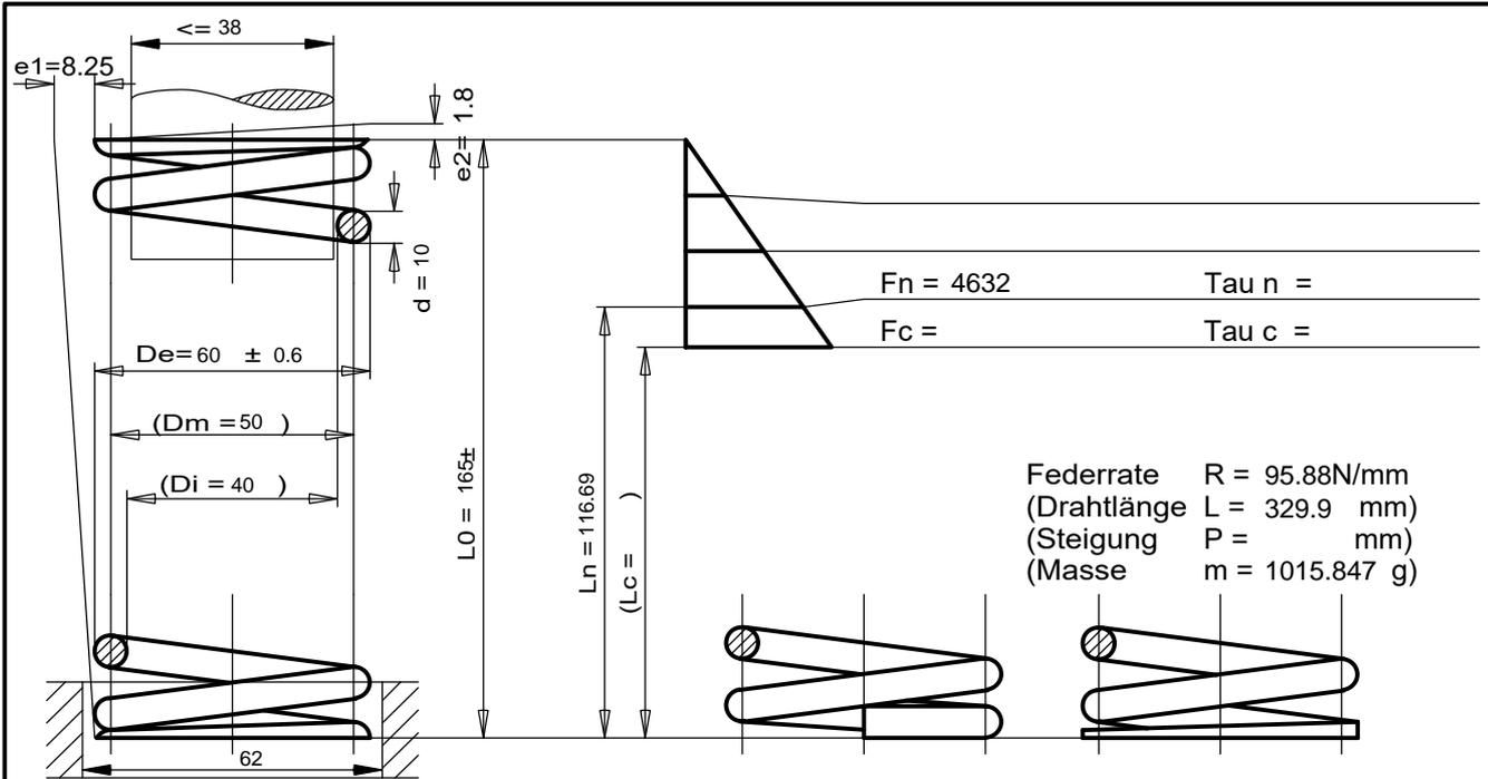
Federrate  $R = 95.88 \text{ N/mm}$
