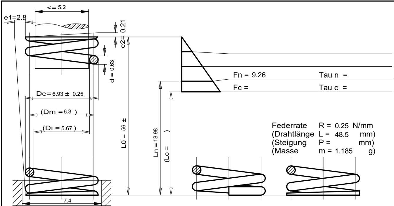
Federrate  $R = 0.25 \text{ N/mm}$
