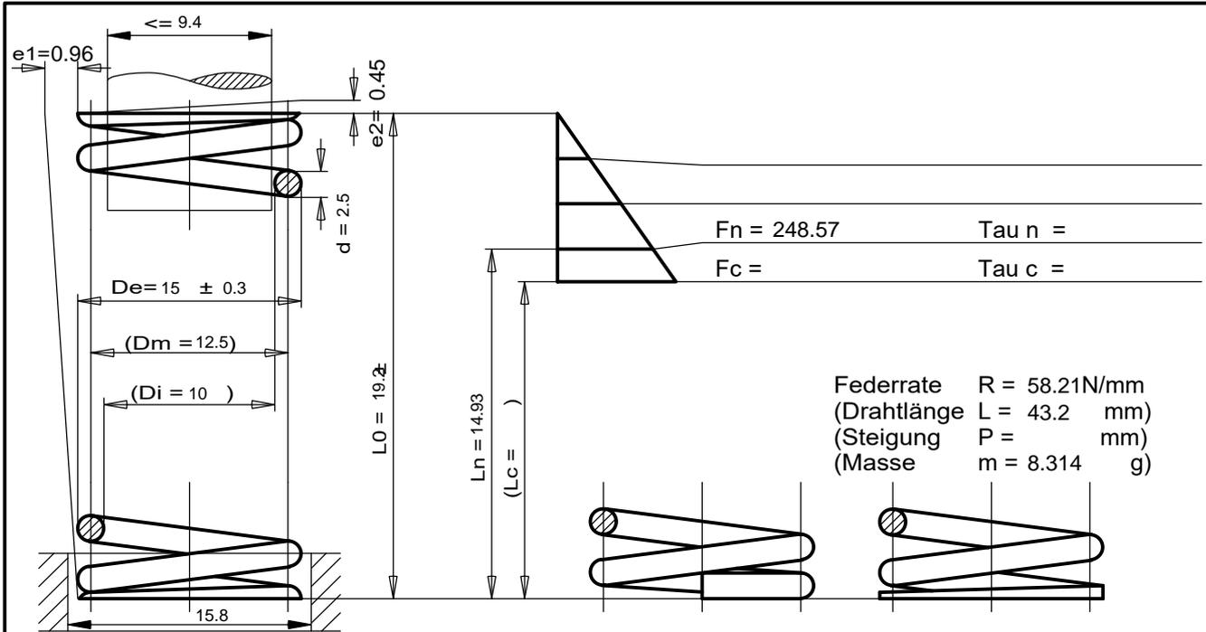
Federrate  $R = 58.21 \text{ N/mm}$
