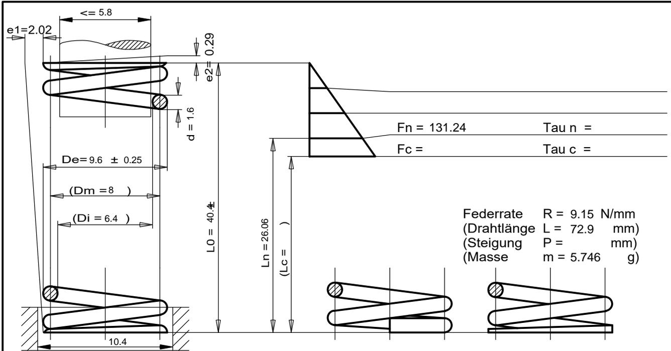
Federrate  $R = 9.15 \text{ N/mm}$
