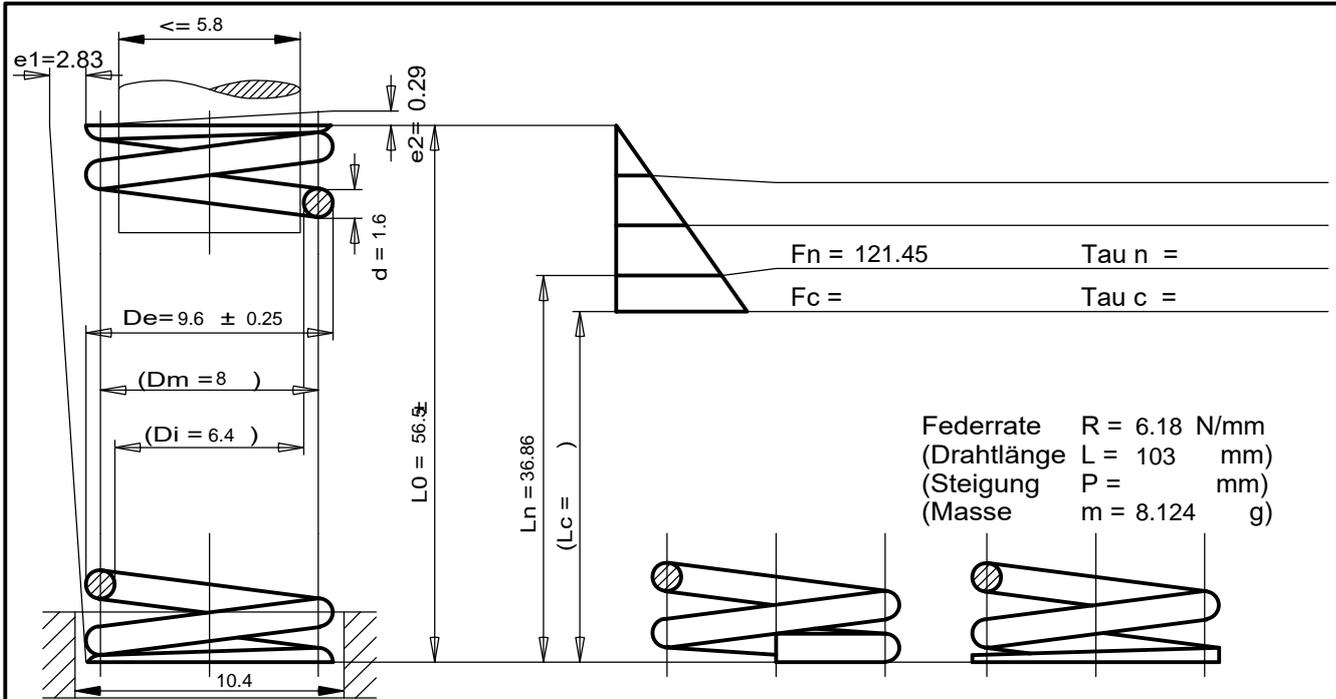
Federrate  $R = 6.18 \text{ N/mm}$
