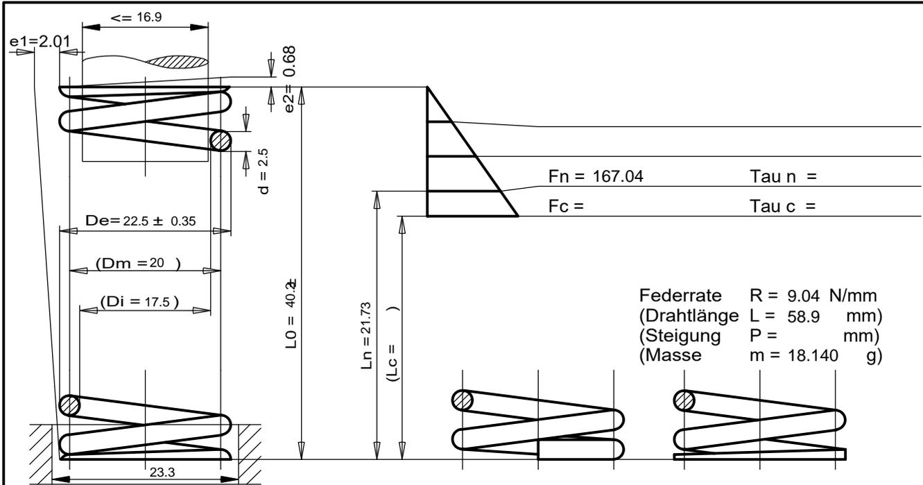
Federrate  $R = 9.04 \text{ N/mm}$
