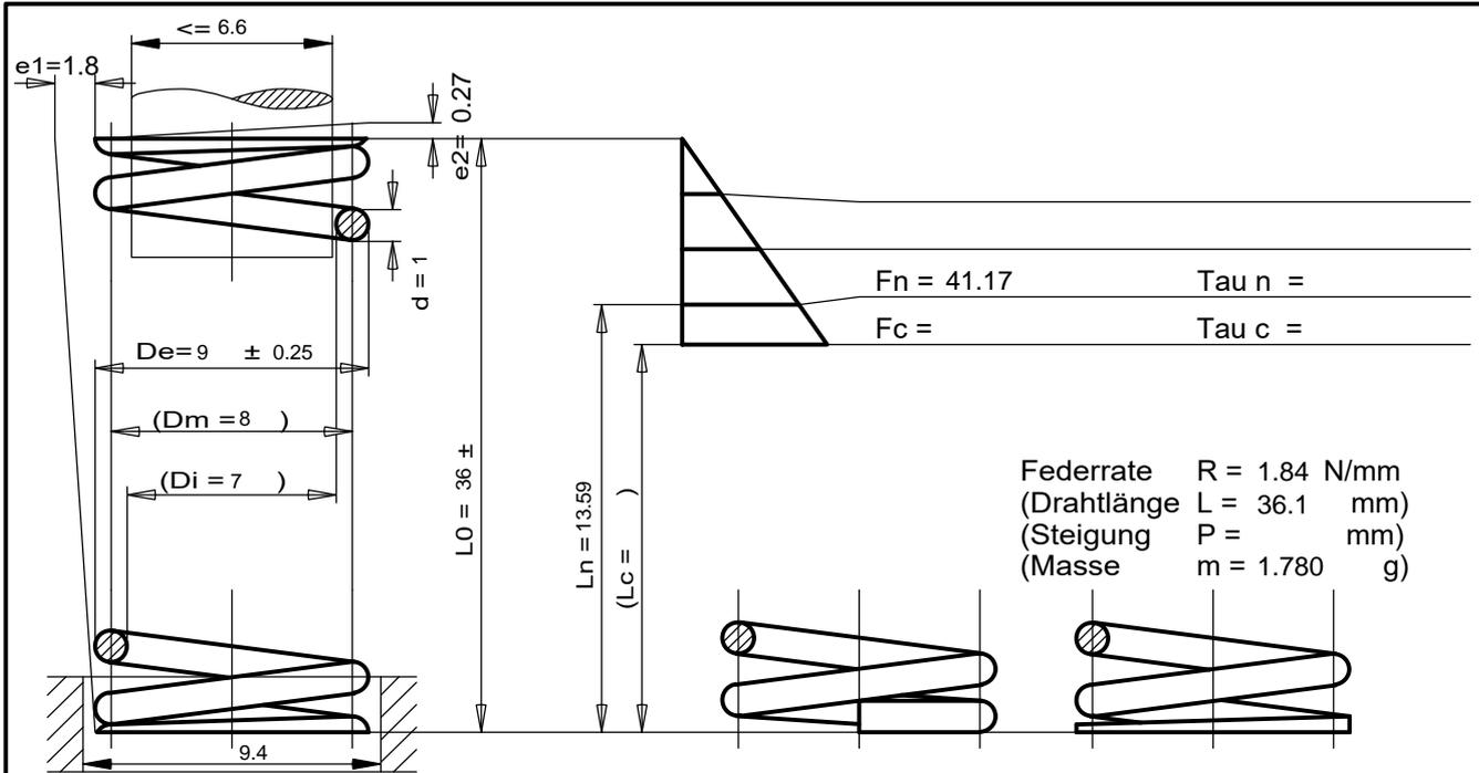
Federrate  $R = 1.84 \text{ N/mm}$
