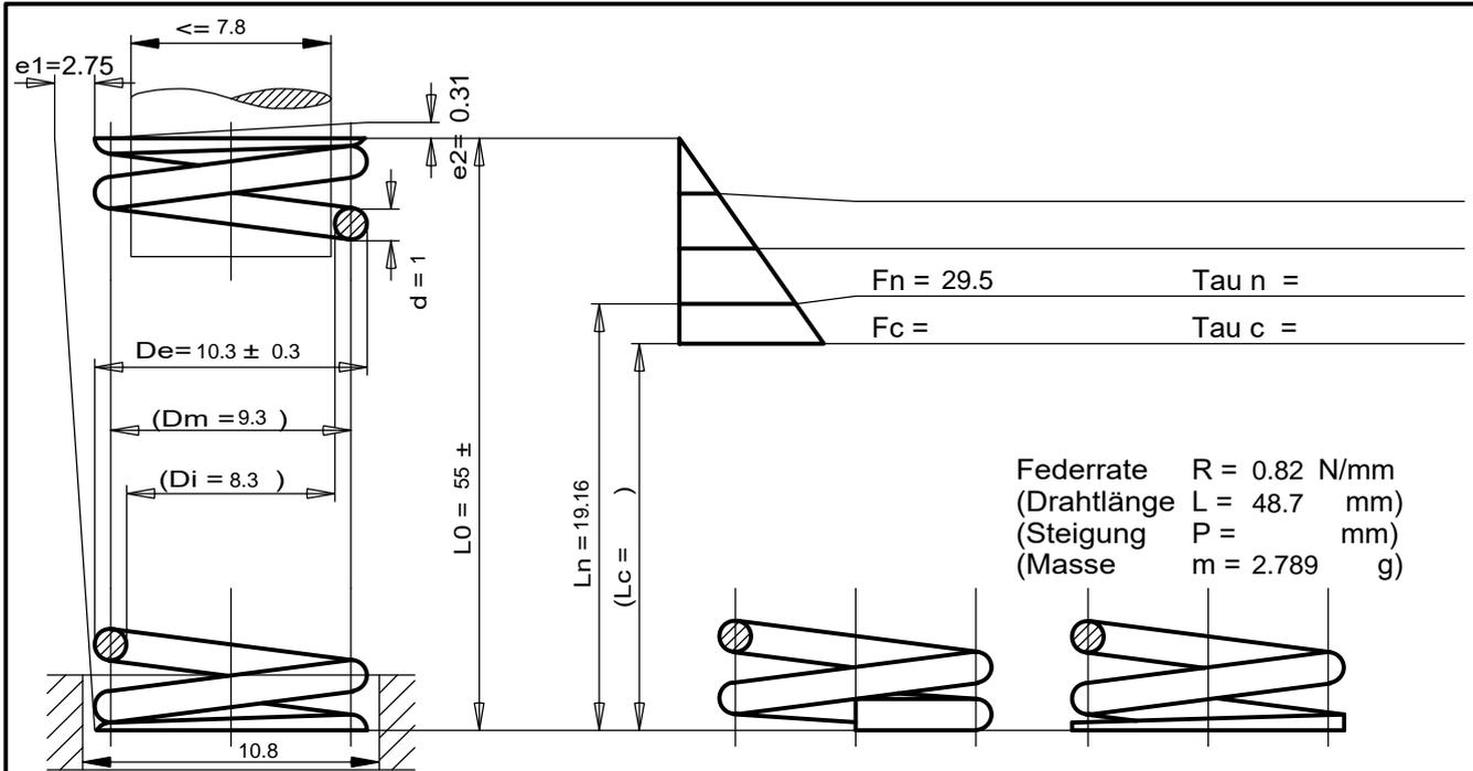
Federrate  $R = 0.82 \text{ N/mm}$
