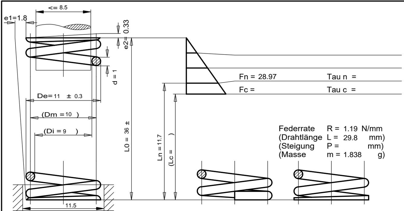
Federrate  $R = 1.19 \text{ N/mm}$
