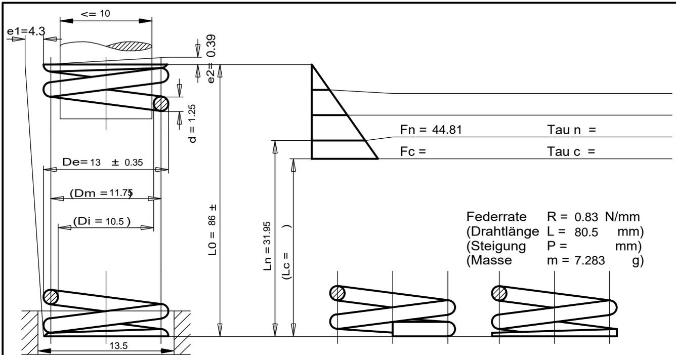
Federrate  $R = 0.83 \text{ N/mm}$
