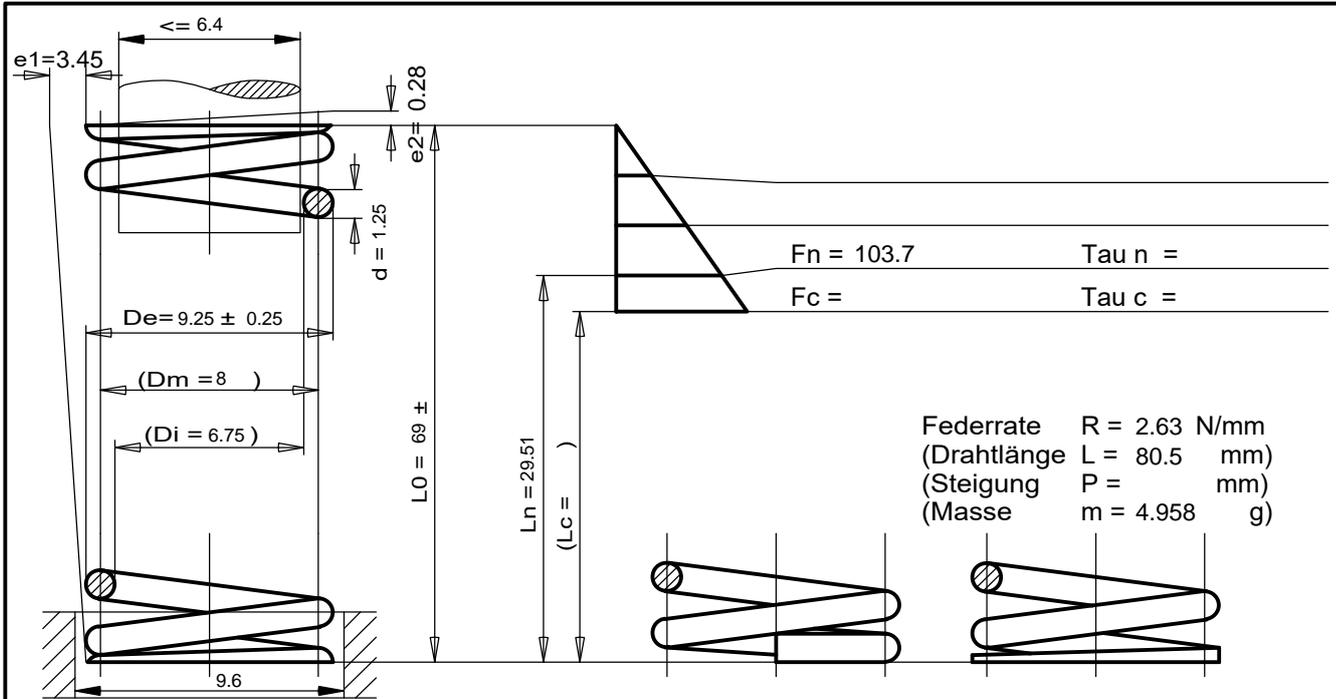
Federrate  $R = 2.63 \text{ N/mm}$
