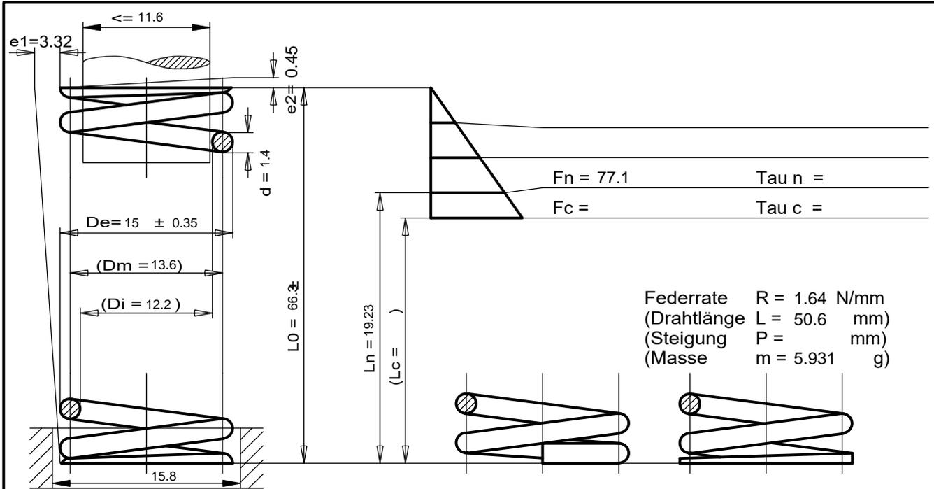
Federrate  $R = 1.64 \text{ N/mm}$
