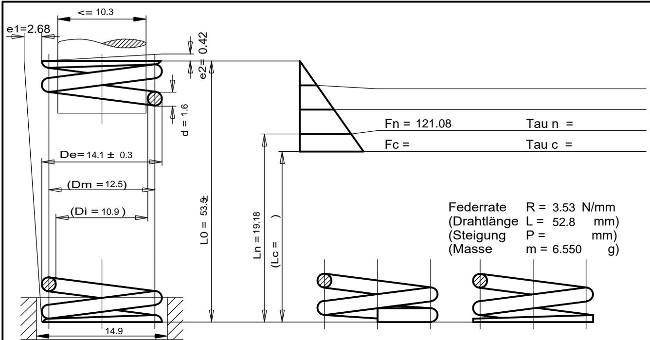
Federrate  $R = 3.53 \text{ N/mm}$
