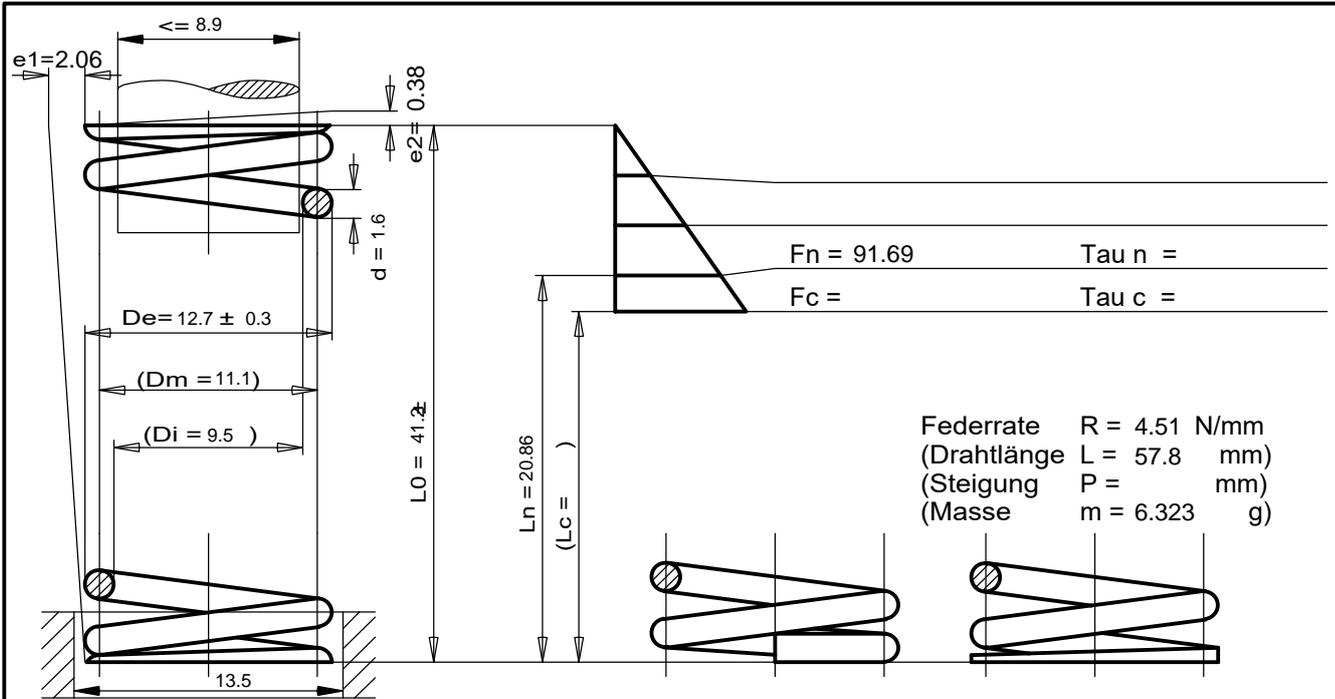
Federrate  $R = 4.51 \text{ N/mm}$
