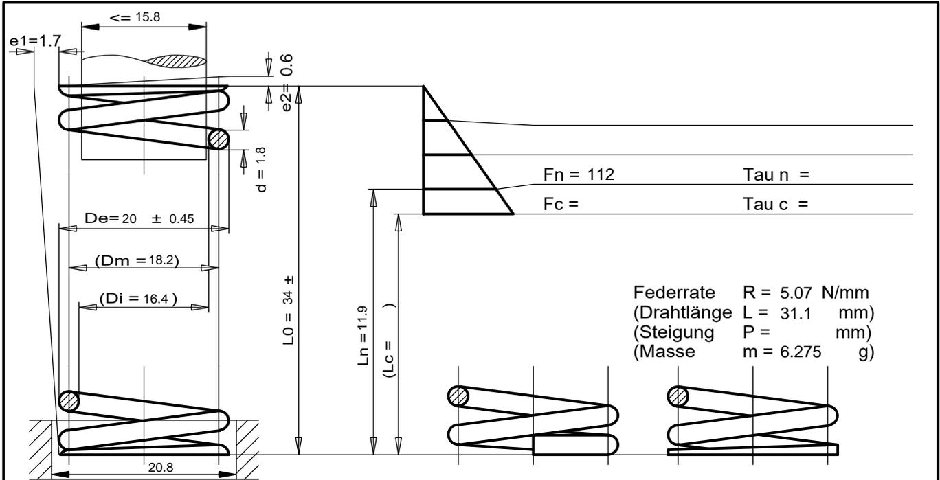
Federrate  $R = 5.07 \text{ N/mm}$
