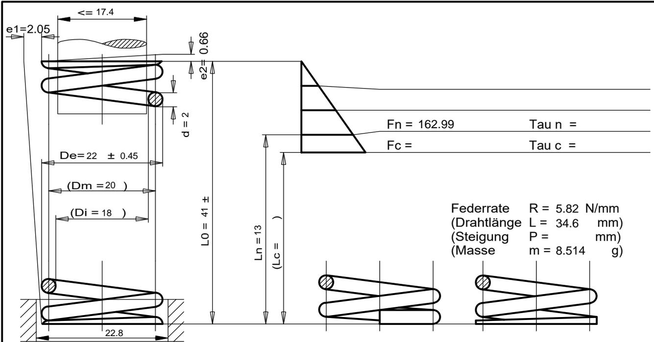
Federrate  $R = 5.82 \text{ N/mm}$
