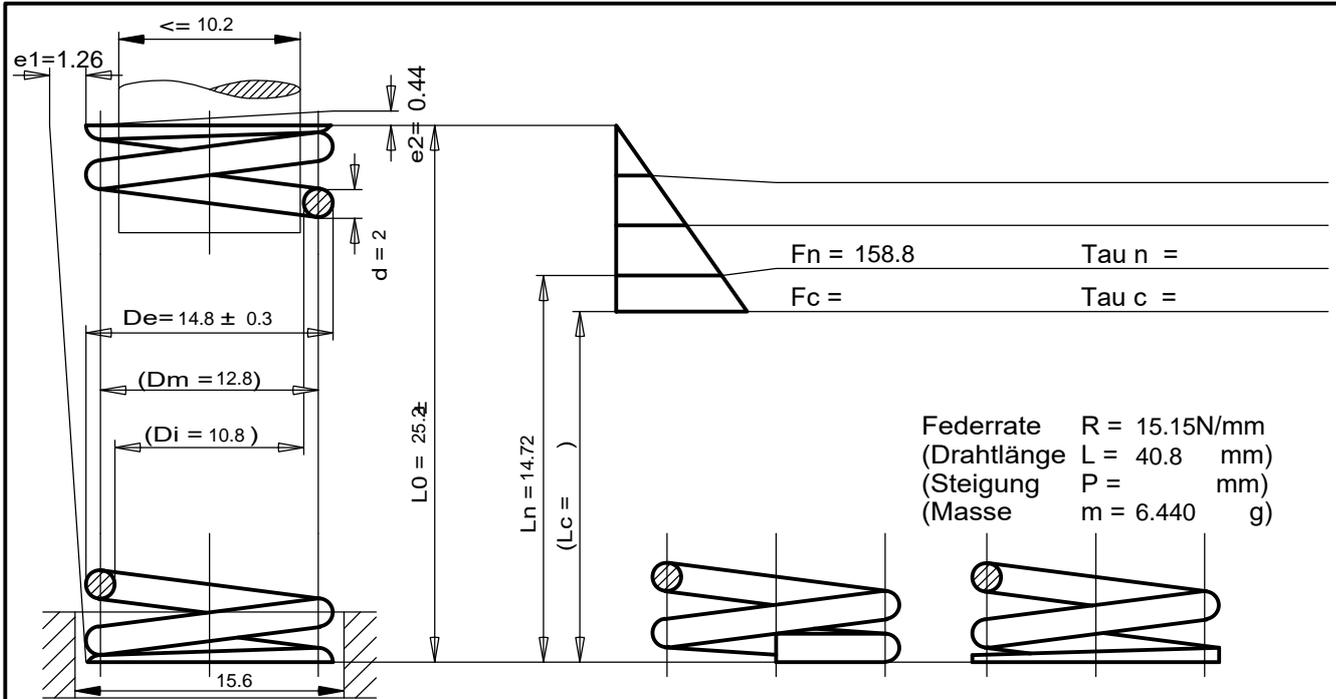
Federrate  $R = 15.15\text{N/mm}$
