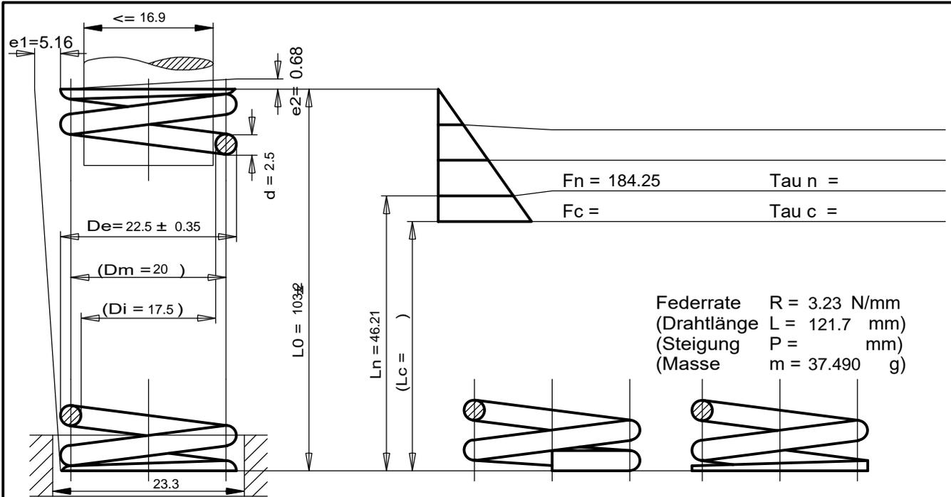
Federrate  $R = 3.23 \text{ N/mm}$
