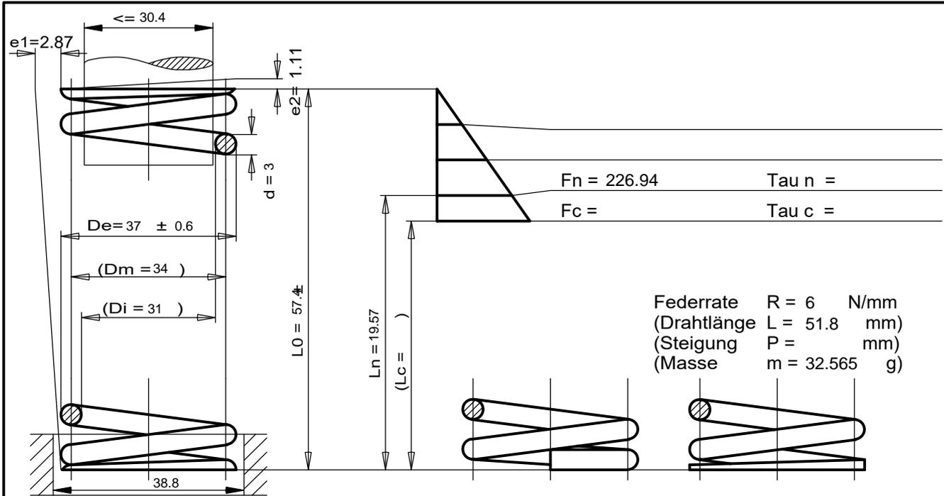
Federrate  $R = 6$  N/mm
