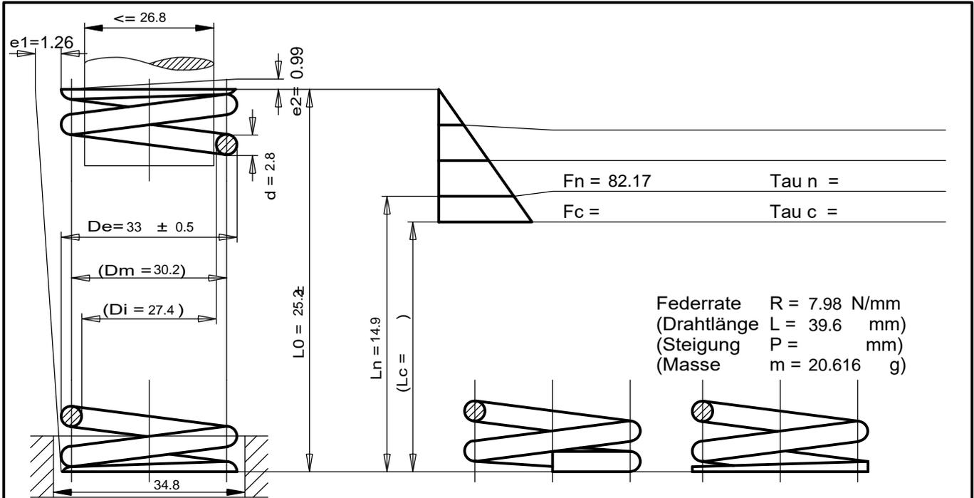
Federrate  $R = 7.98 \text{ N/mm}$
