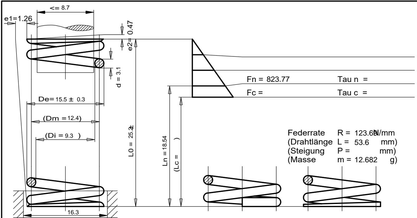
Federrate  $R = 123.6 \text{ N/mm}$
