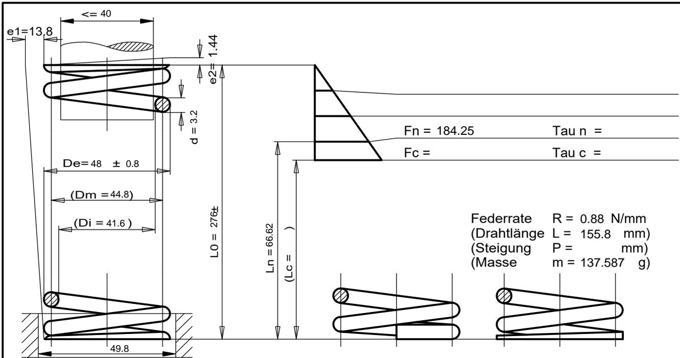
Federrate  $R = 0.88 \text{ N/mm}$
