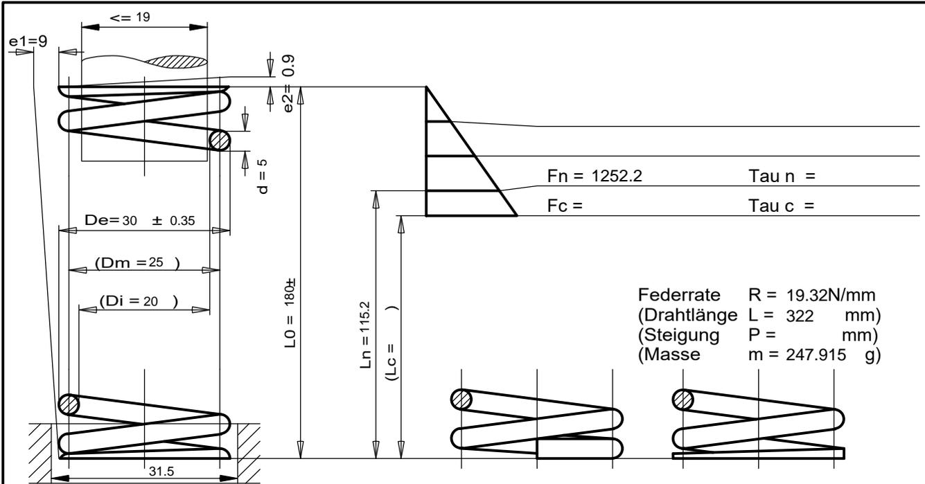
Federrate  $R = 19.32\text{N/mm}$
