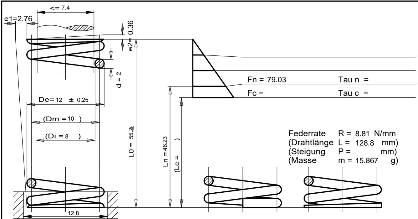
Federrate  $R = 8.81 \text{ N/mm}$
