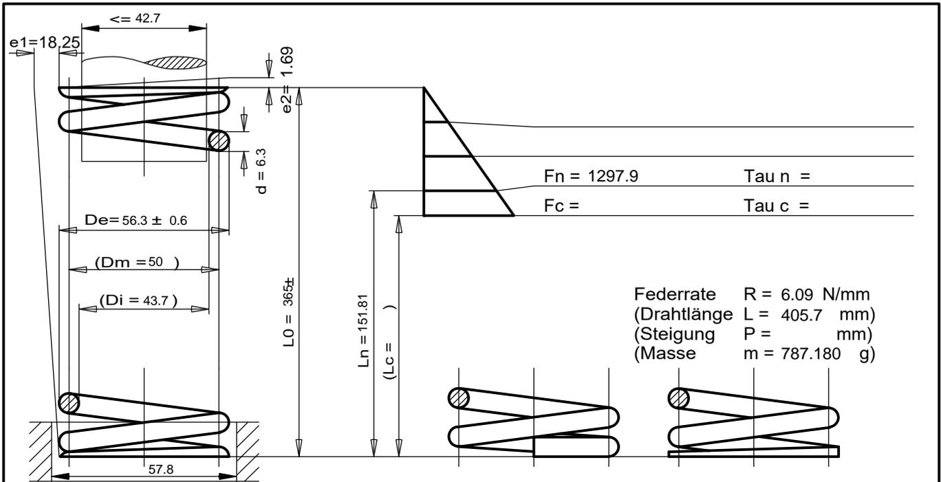
Federrate  $R = 6.09 \text{ N/mm}$
