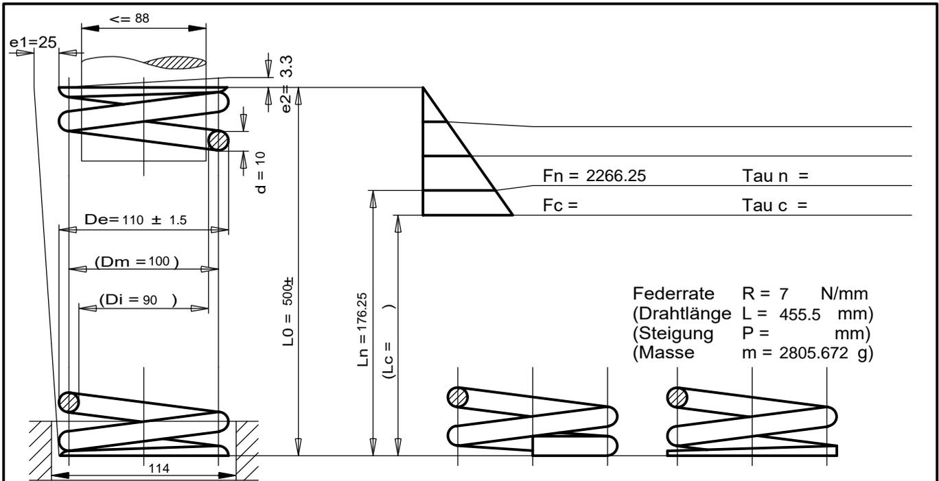
Federrate  $R = 7$  N/mm
