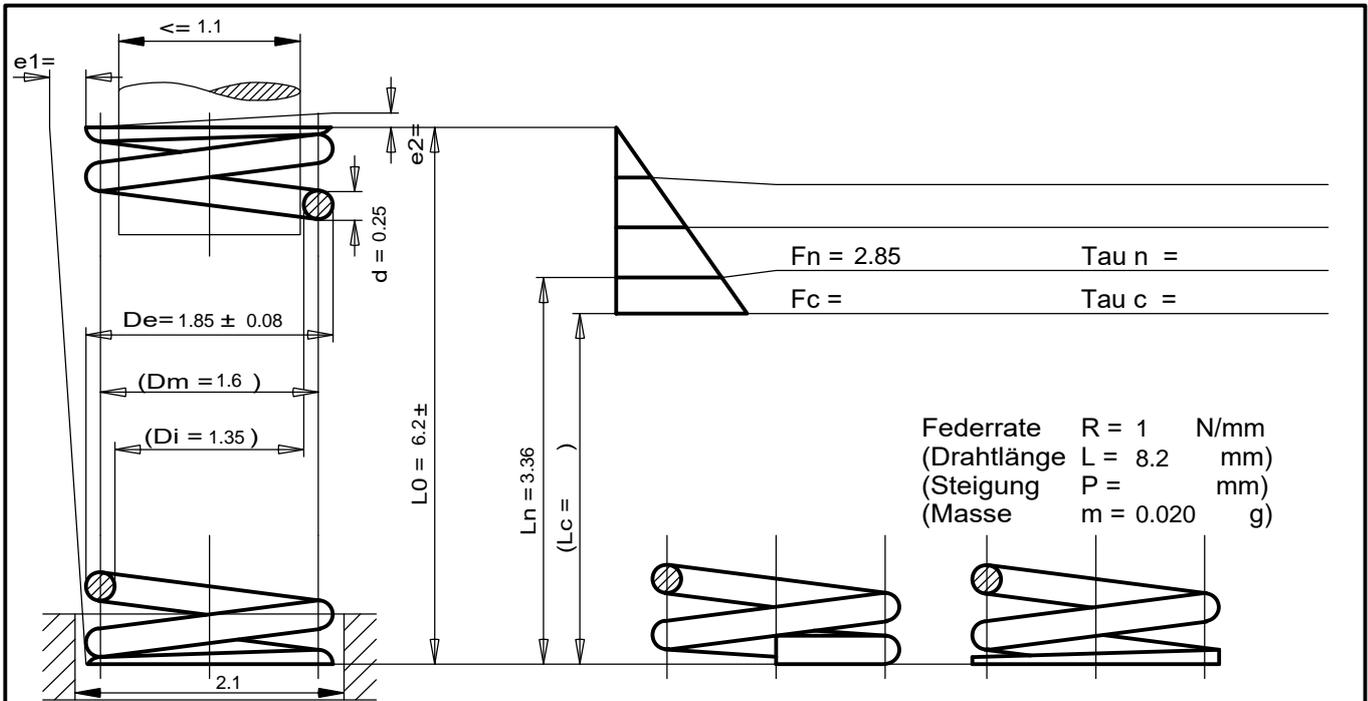
Federrate R = 1 N/mm
