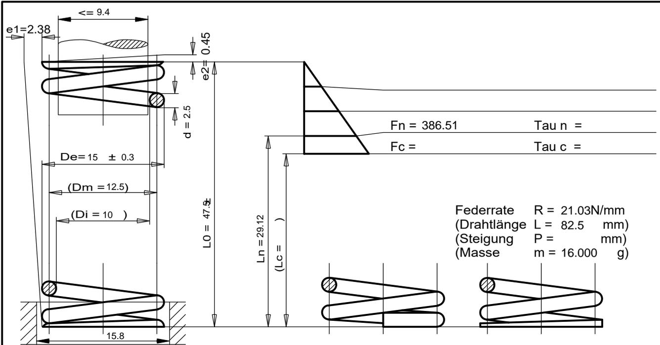
Federrate  $R = 21.03\text{N/mm}$
