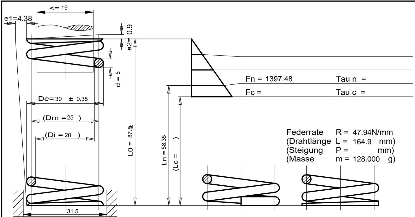
Federrate  $R = 47.94\text{N/mm}$
