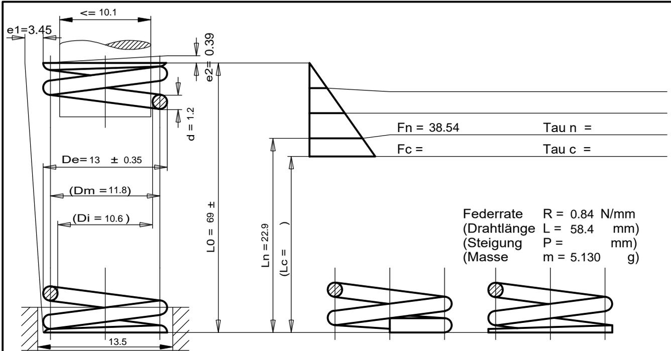
Federrate  $R = 0.84 \text{ N/mm}$
