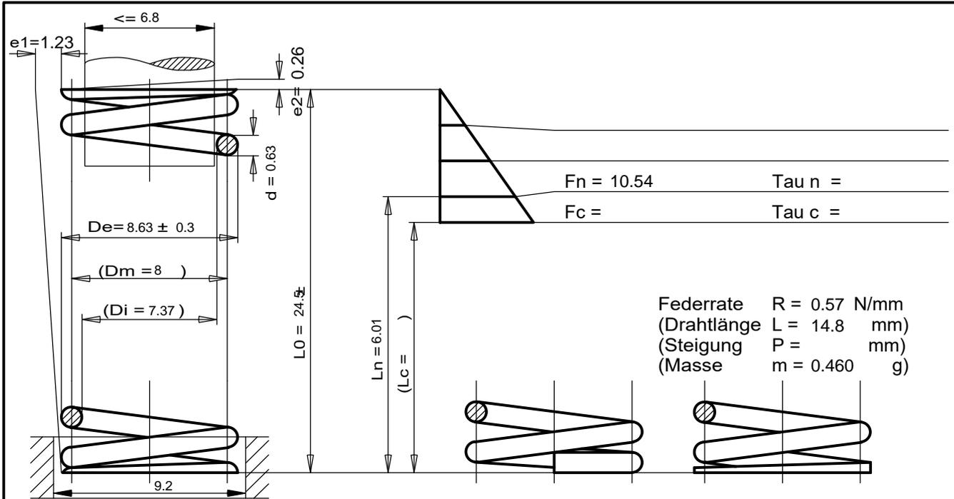
Federrate  $R = 0.57 \text{ N/mm}$
