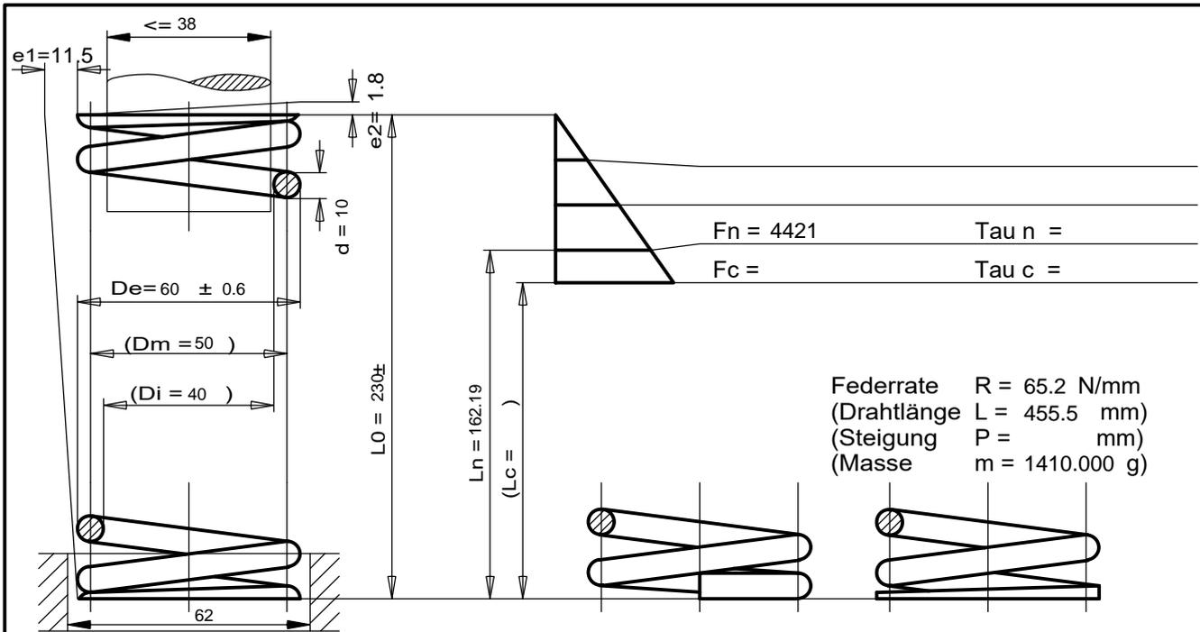
Federrate  $R = 65.2 \text{ N/mm}$
